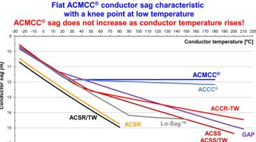
Due to the application of annealed AL wires, the ACMCC® conductors' so called knee point occurs at a low temperature while due to the application of a carbon fibre core, the sag curve remains almost flat as the temperature rises. In the case of conductors with a polymer composite core but with hard drawn aluminium zirconium alloy ALZr wires, the knee point is located at much higher temperatures, whereby their sag is by 1-2 meters larger than that of ACMCC® conductors.
