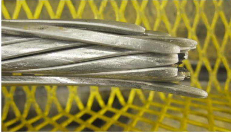
Figure 7 Magnified View of Conductor Aluminum Strands at Breaking Point
