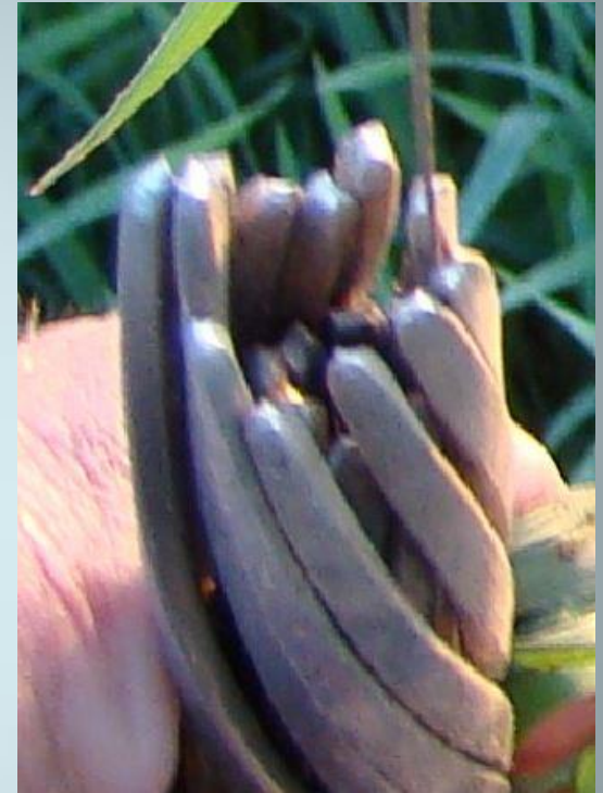
Figure 7 Magnified View of Conductor Aluminum Strands at Breaking Point
